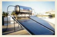
Capacity: 100 to 500 LPD This model is recommended in house where the over head tank is at a very high level or a pressure booster pump is installed. Celesti has a greater pressure withstanding capacity with its heavy-duty tank and can operate at pressure ranging between 2.0 and 6kg/cm2, custom designed tank to operate with much higher pressure also can be designed. These systems are provided with pressure and vaccum relief value
